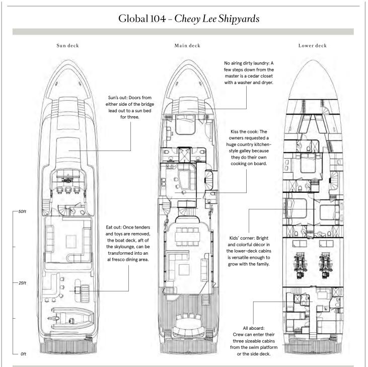
LOA: 103' 10" (31.7m) Beam: 22' (6.7m) Draft: 5' 10" (1.8m) Displacement: 211,500 pounds Power: 2 x 1,900-hp Caterpillar C32 ACERT Speed (max/cruise): 25.8/22 knots Range: 2,400 nm @ 11 knots Fuel capacity: 5,000 U.S. gallons Stabilizers: Naiad Generators: 2 x 55kW Kohler Thrusters: Naiad Freshwater capacity: 600 U.S. gallons Black/gray water capacity: 350 U.S. gallons each Owner and guests: 10 Crew: 5 Construction: FRP Naval architecture: Jon Overing Interior design: Sylvia Bolton
